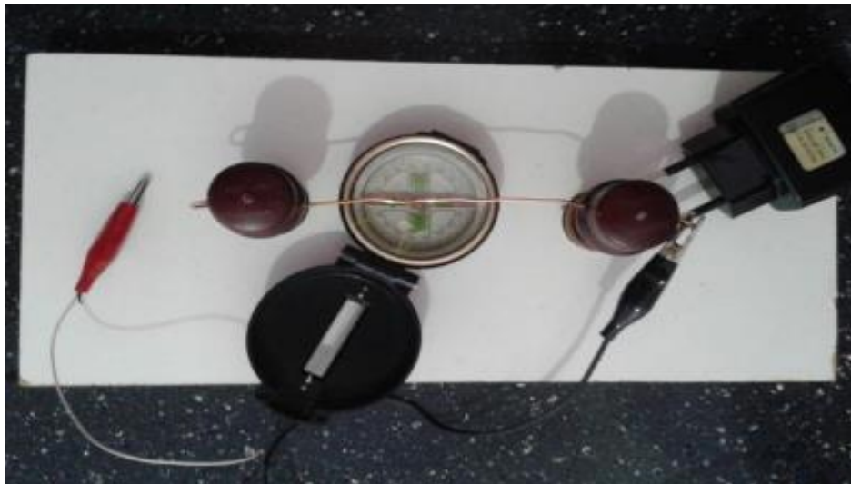
Figura 3 – Experimento de Oersted
