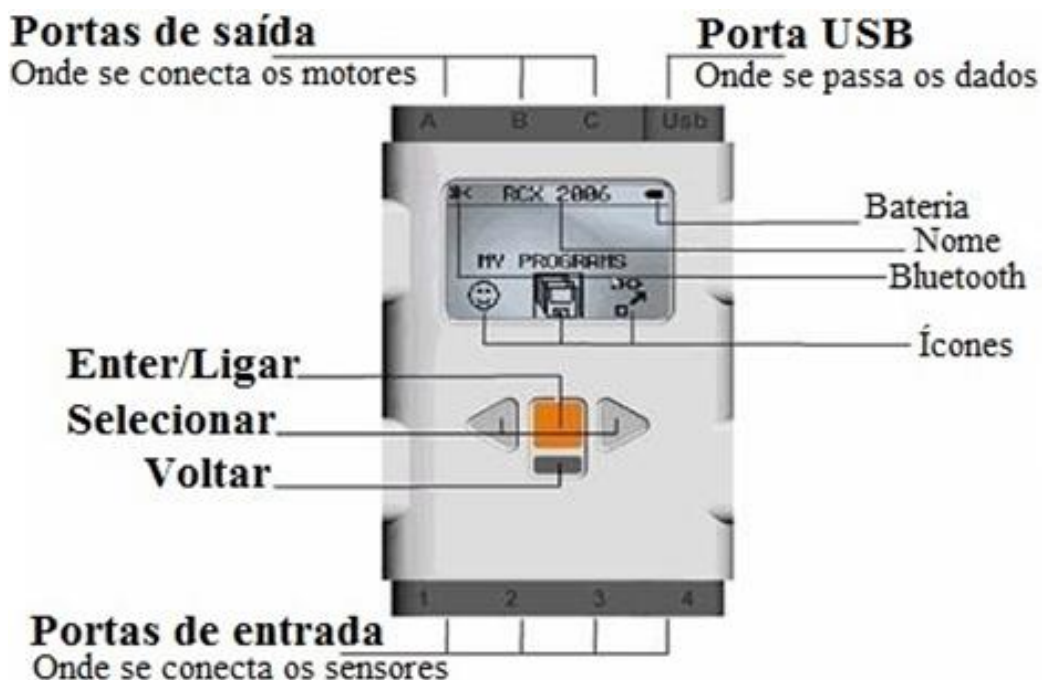
Figura 4 - NXT Intelligent Brick
