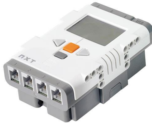
Figura 2 - NXT Intelligent Brick
